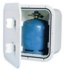
For 3 kg bottles, fitted with respective pressure regulator. Product includes UV-resistant Luran hatch and watertight gas hose joint. In compliance with ISO 10239 standard. Remote ventilation by means of 16-mm Ø hose.
