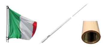
VHF antenna featuring an innovative design where the built-in bushing perfectly matches the boat look. Fitted with flag holder at the end. 2.4-m long. 6-db gain, 100W max. applicable power. Fitted with RG58 6-m cable. Recommended base 29.133.00.
