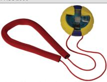
Compass fitted with **rubber** anti-shock housing. BETA ray permanent lighting. Magnifying lens for use as both bearing compasses and steering compasses. It uses the twenty-year-old unmatched **direct vision** system without lubber lines. The rose image is enlarged **10 times**; no parallax, 0.5° interval estimate. Excellent rose stability and quickness.
