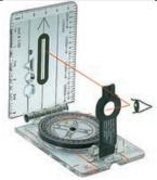
$\label{liquid-filled} \mbox{Liquid-filled compass with } \mbox{{\bf rotating} rose, scale meter and foldable sight frame.}$
