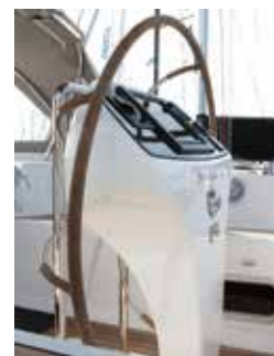
Custom dish wheel designed to mount on the back face of the customer's own pedestal for which they have a registered trademark.
